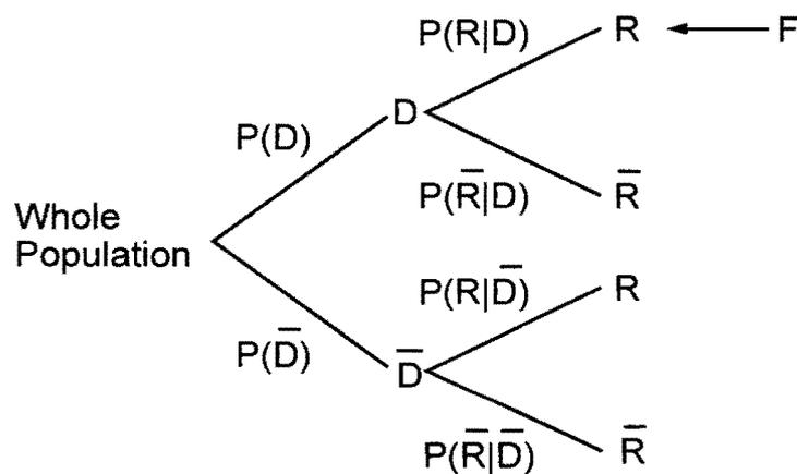
The probability of ending up in group F is precisely  $P(R \cap D)$  and it is clear from the branching diagram that conditional probabilities multiply
