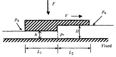
a) In a frame of reference moving with the bearing, sketch the velocity profiles in the left and right halves of the bearing, far from the region close to the step.
