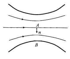
a) Along the narrowest section, AB, where will the pressure be lowest and where will it be highest?
