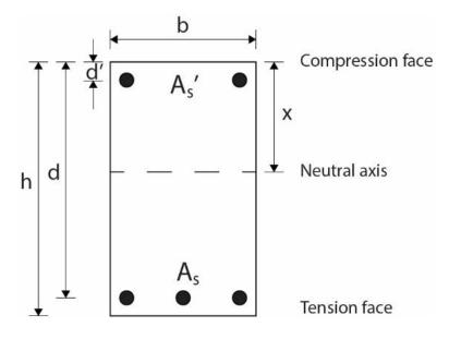
Design compressive strength of concrete is based on the characteristic cylinder strength  $f_{ck}$ :  $f_{cd} = \alpha_{cc} \frac{f_{ck}}{1.5}$
