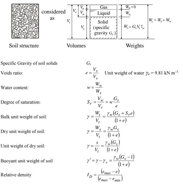
where:  $e_{max}$  is the maximum voids ratio achievable in a quick tilt test, and  $e_{min}$  is the minimum voids ratio achievable by vibratory compaction.
