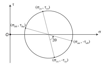
The stresses on perpendicular faces,  $(\sigma_{xx}, -\tau_{xy})$  and  $(\sigma_{yy}, \tau_{yx})$ , plot at the opposite ends of a diameter. If new faces are considered at angle  $\theta$  (see Section 2.5), the stresses on the new faces can be obtained by rotating the diameter of Mohr's circle by  $2\theta$  in the same direction.
