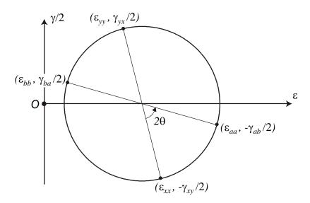
The strains in perpendicular directions,  $(\varepsilon_{xx}, -\gamma_{xy}/2)$  and  $(\varepsilon_{yy}, \gamma_{yx}/2)$ , plot at the opposite ends of a diameter. If new faces are considered at angle  $\theta$  (see Section 2.7), the strains in the new directions can be obtained by rotating the diameter of Mohr's circle by  $2\theta$  in the same direction.
