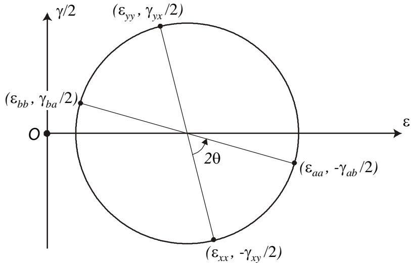
The strains in perpendicular directions,  $(\epsilon_{xx}, -\gamma_{xy}/2)$  and  $(\epsilon_{yy}, \gamma_{yx}/2)$ , plot at the opposite ends of a diameter. If new faces are considered at angle  $\theta$  (see Section 2.7), the strains in the new directions can be obtained by rotating the diameter of Mohr's circle by  $2\theta$  in the same direction.
