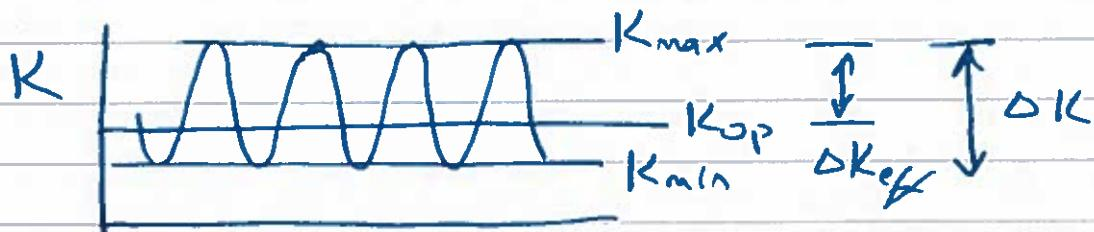
Fatigue crack growth is driven by  $\Delta K_{eff} = K_{max} - K_{op}$
