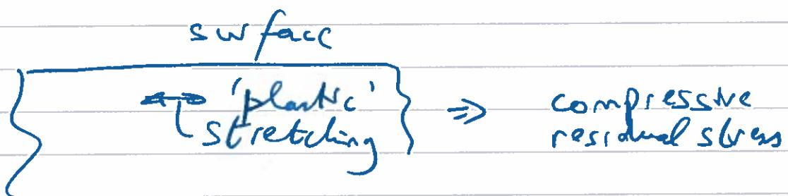
Compressive stresses delay crack initiation (recall the Goodman correction) and lead to a lower R-value, hence retarded da/dN.
