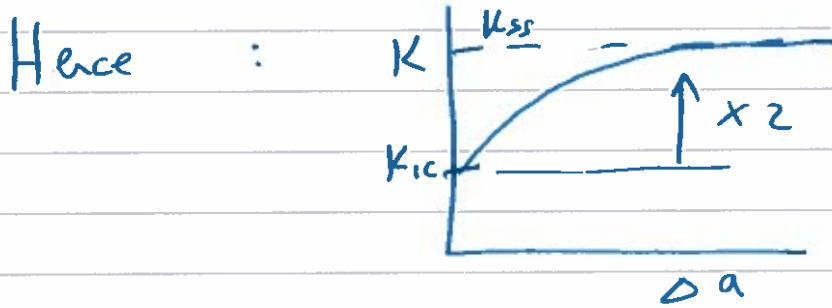
The thickness of the plate dictates the level of hydrostatic stress: plastic constraint raises the hydrostatic stress and lowers the R-curve for a thick specimen.
