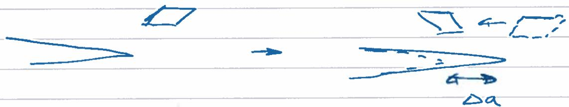
As the crack advances, material is sheared in one direction and then back in the opposite direction, and plastic hysteresis occurs.
