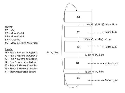
Note that Robot 1 has four potential outputs so cannot be treated as a simple on/off device.
