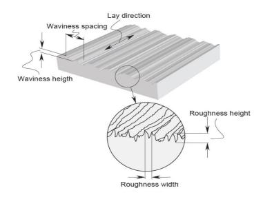
Surface finish is characterised by the following parameters: <u>Roughness:</u>
