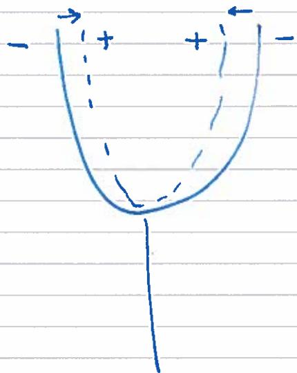
The prongs move in and out in a symmetric motion. The motion of each prong creates a dipole. The two dipoles are out of phase, leading to a longitudinal quadrupole.
