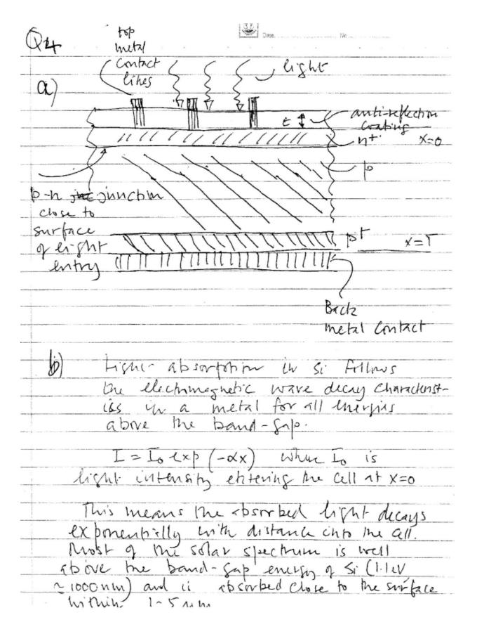
The protection of agreening a photon electron-hole pair ted a photo convent- and vollage decays exponentially away me dipletion edge of the B-h on. Therefore the junction to placed these to the surface where most of the solar spectrum absorbed 10 m3 Solar photon witchus as Tak 10 m depletion refin 511 Probability ex Collection 1/e This requires the junction to be placed Clove to the & surface. thousever, this then poses he problem of electrons in the h-layer hing to trans
