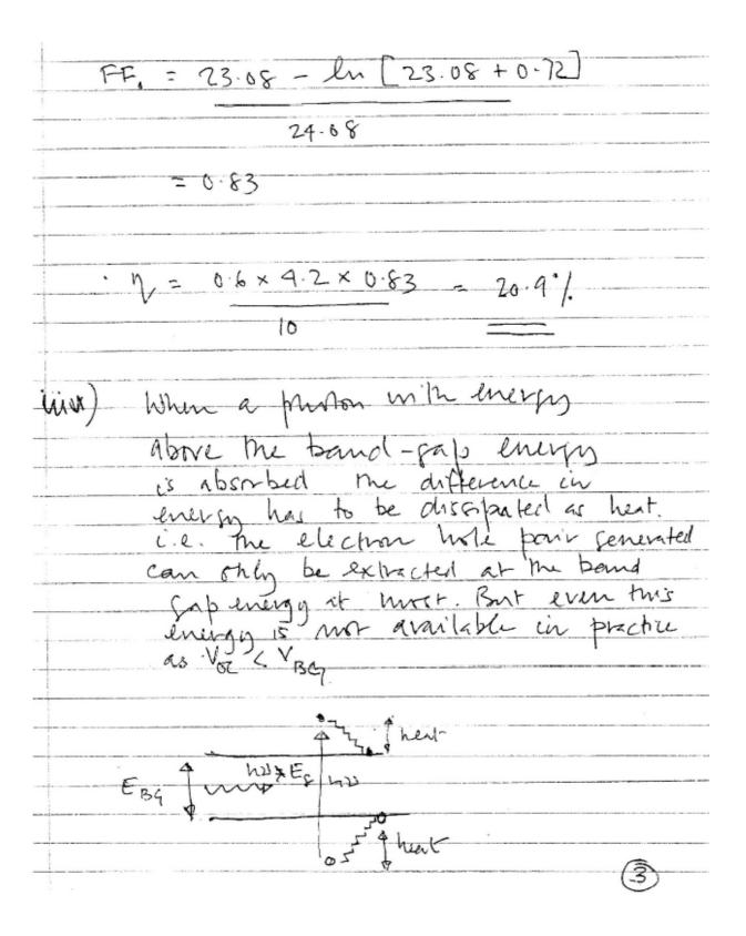
Therefore the Solar Cell in operation will get hot and be above the ambient (dark) temperature. It has to be in equitionium with the environment, can's mens it will test a temperature above antiment which allows it to maintain a tadiative heat flux out of it which is equal to the heat dissipated by the absorbed ponotons. If temperature vises then his will vise.
