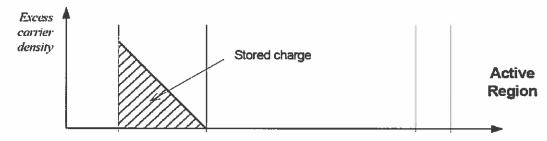
Deep saturation or 'hard saturation' region. Both BE and BC junctions are forward biased. The charge is stored in the base and the collector region. In deep saturation the plasma level is very high and the charge reaches the other side of the collector (where the n+ contact is). This regime is good for on-state but switching losses could be high as the deep plasma slows down the device during turn-off.
