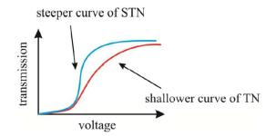
The STN device was preferred to the TN mode in passive matrix addressed LCDs, however the steep transmission curve means that the control of grayscale is difficult. STN failed for two main reasons: 1) The viewing characteristics were much worse than the TN due to this higher twist. 2) As active matrix backplanes became better and cheaper it became unnecessary to rely on passive matrix displays and so the better viewing characteristics of the TN could be used a high levels of multiplex.
