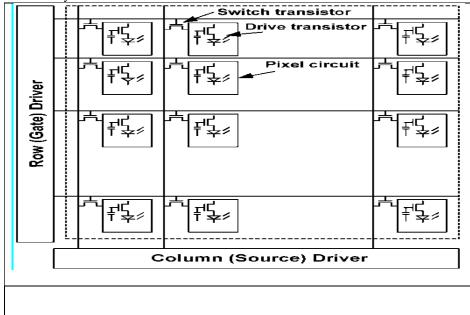
The driver diagram for the LCD should be similar to that of the OLED array except that the drive transistor and diode is now replaced by the liquid crystal capacitance. There should be a clear definition between the current drivers needed for the OLED array as opposed to the electric field (or voltage drivers required for the LCD)
