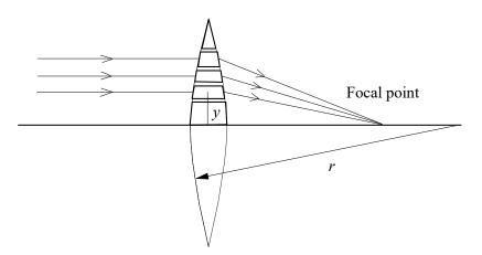
The deviation of each ray means that if parallel rays are incident on the lens, then they will all converge to the same point called the focal point or focal length of the lens. This relationship forms the basis of most geometrical optical systems and is one of the fundamental relationships which are exploited on a regular basis in optical design procedures.
