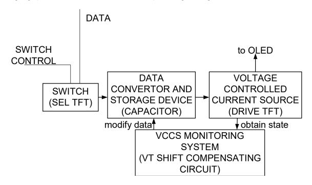
Rightmost and lower blocks highlight the fundamental differences in terms of backplane requirements between the AMOLED and AMLCD.
