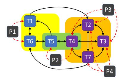
c) The DSM (bottom right) should be filled in, taking note of the links between tasks and people from part b). In particular, person 1 performs tasks 1 and 6 without interaction with any other person. Persons 2, 3, and 4 interact on tasks 2-5 and 7. This is easier to see if part a) is completed correctly, but could also be spotted from the original MDM. A possible DSM configuration is:
