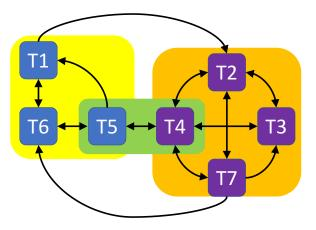
The task to person Domain Mapping Matrix (DMM) interactions are added to the diagram. The task to person interaction arrows should be clearly different from the task to task arrows.
