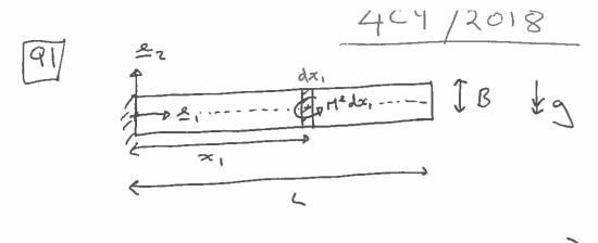
(a) Diploment field:  $\underline{u} = w(z_1) \underline{z}_2 - \frac{\partial w}{\partial z_1} z_2 \underline{z}_1$
