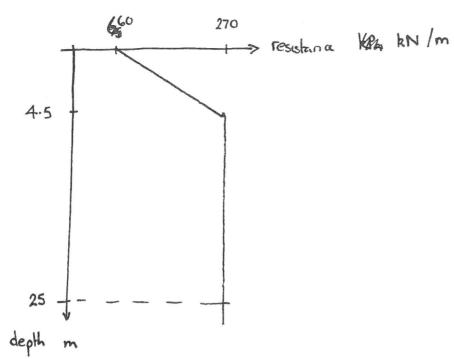
b) Pile restrained at head no bending failure so pile translates through soil
