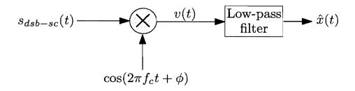
Show that the demodulated signal is  $\hat{x}(t) = x(t) \cos \phi$ . What happens when  $\phi = 90^{\circ}$ ?
