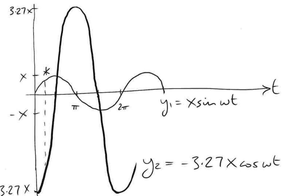
c) collision if  $|y_1 - y_2| = 10 \text{ mm}$  (AT ANY TIME)
