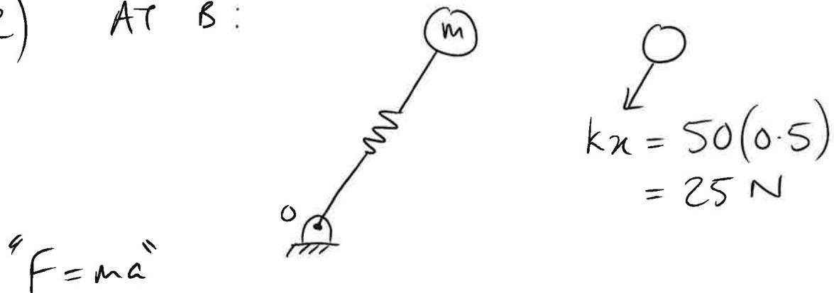
$$\therefore a_B = \frac{25}{1.5} = \underline{\underline{16\frac{2}{3} \text{ m/s}^2}} \quad (\text{NORMAL TO VELOCITY VECTOR})$$
