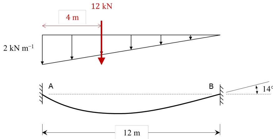
Flexible cable so cannot sustain bending moments, statically determinate so solve by equilibrium. Taking moments about A:
