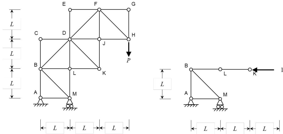
a) Statically determinate truss structure. By equilibrium and free-bodies (method of joints and/or sections), or graphically, we obtain column 2:
