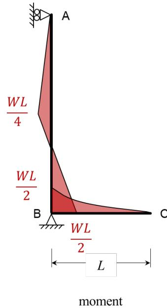
b) By superposition of databook cases, considering the effects of: the anti-clockwise rotation at B due to the point load; the clockwise rotation of B due to the distributed load, and the bending of BC due to the distributed load:
