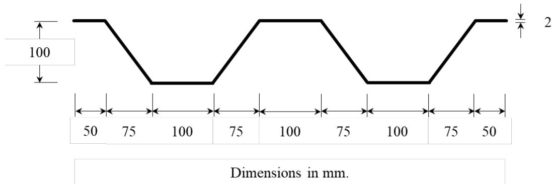
Horizontal distribution of material does not affect the second moment of area about the horizontal neutral axis. So, the inclined webs can be converted to equivalent vertical webs of the same height but with a commensurately increased thickness of 2.5 mm.
