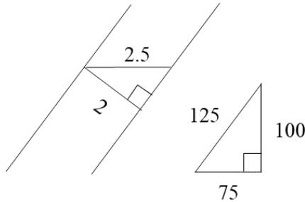
The second moment area of the section is then most easily calculated as that of an equivalent box section:
