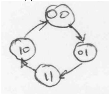
$$\begin{aligned} Q_2^+ &= Q_1 \\ Q_1^+ &= \bar{Q}_2 \end{aligned}$$
