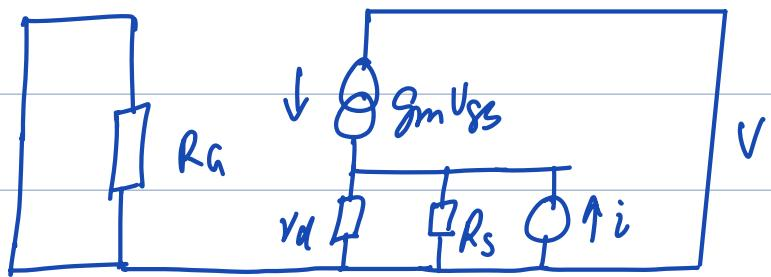
$$(i + g_m V_{GS}) (R_s \parallel r_d) = V = -V_{GS}$$
