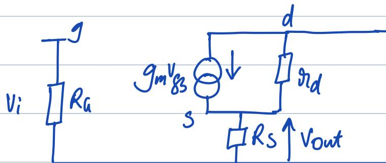
$$V_{out} = g_m V_{gs} (R_s \parallel r_d)$$
