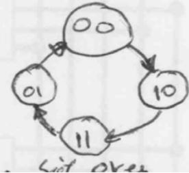
(b) This is a Grey code, in which only one bit changes at a time. It is used in sequential logic applications where dynamic hazards must be avoided
