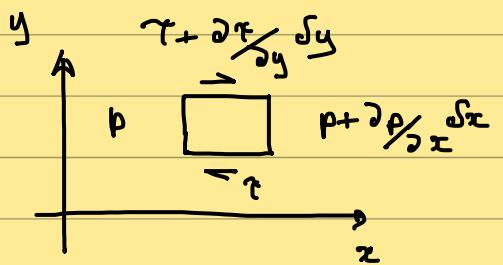
$$p \cancel{\delta y} - \left( p + \frac{\partial p}{\partial x} \delta x \right) \delta y - \cancel{v \delta x} + \left( v + \frac{\partial v}{\partial y} \delta y \right) \delta x = 0$$
