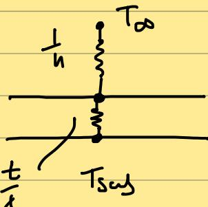
$$\frac{q}{A} = \frac{T_{\infty} - T_{\text{solid}}}{\frac{1}{h} + \frac{1}{\lambda}}$$
