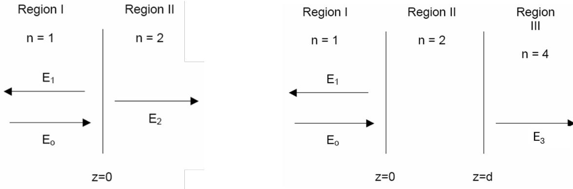
Since  $\theta_i = 0^\circ$ , let's write down all the reflection and transmission coefficients:
