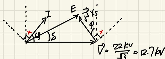
Star connection,  $I_{ph} = I_{line} = 7873 \text{ A}$
