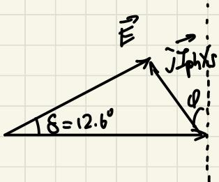
$$I_{ph} \times_s \cos \phi = E \cdot \sin \theta = 2.26 \text{ kV}$$
