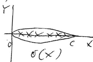
Thickness represented by a source distribution,  $\sigma$ , source/length
