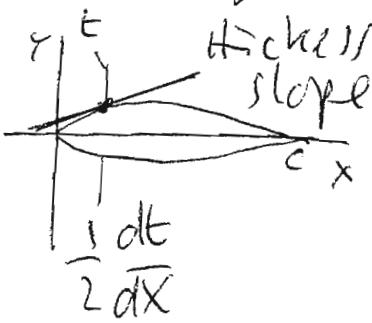
physically we match the local streamlines to the "thickness slope"
