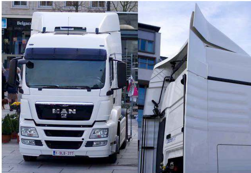
Tractor-trailer gap treatment
