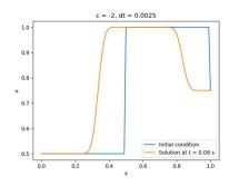
The artificial viscosity term is now important and the profiles are smudged as they are convected.
