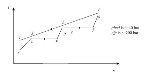
Saturation temperature at 200 bar is 365.75 °C.
