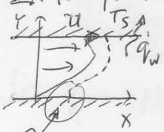
$$\alpha \frac{dT}{dy} = \left(\frac{dT}{dx}\right) \left\{ \frac{Uy}{H} + \frac{1}{\mu} \left(\frac{dp}{dx}\right) \frac{1}{2} \left( \frac{y^3}{3} - Hy^2 \right) \right\} + A$$
