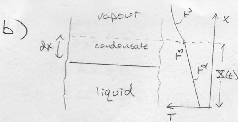
$$\dot{q}_{\text{cond},v}'' = \dot{q}_{\text{cond},l}'' + \dot{q}_{\text{latent}}''$$
