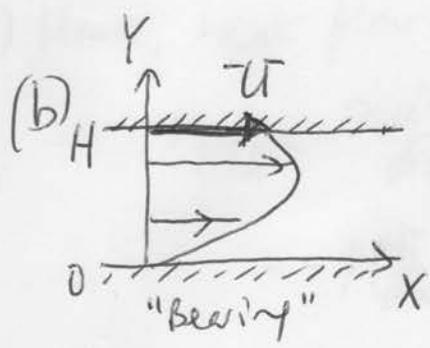
fully developed, steady, laminar flow:
