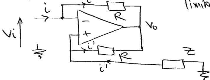
$$V_- = V_i = V_+ \\ i' = i \\ \therefore Z_{in} = \frac{V_i}{i} = -Z$$
