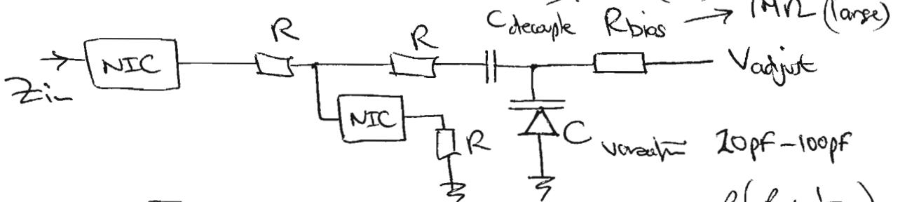
$$Z_{in} = - \left[ R + -R \parallel R + \frac{1}{j\omega e} \right] = - \left[ R + \frac{-R(R + \frac{1}{j\omega C})}{-R + R + \frac{1}{j\omega C}} \right] \\ = - \left[ R - R^2 j\omega C - R \right] = j\omega C R^2 = j\omega L$$
