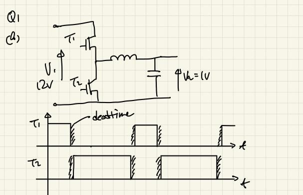
(ط To has borrer switching loss. The borg diale of To conducts connect during deattine. Therefore, When T2 surides on after the deadtime, it has vearly zero where and the suitching on loss is hearly zero.
