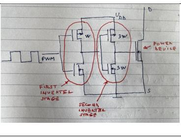
The two-stage inverters are typical CMOS with a n-channel on the low side and p-channel on the high side. The second inverter has larger transistors (e.g. 3x width or even larger) to minimise the on-state resistances of the n-channel and p-channel transistors. The gate resistance is not specifically shown, but could be internal or added between the output of the second stage and the gate of the power transistor to control the dVdt.
