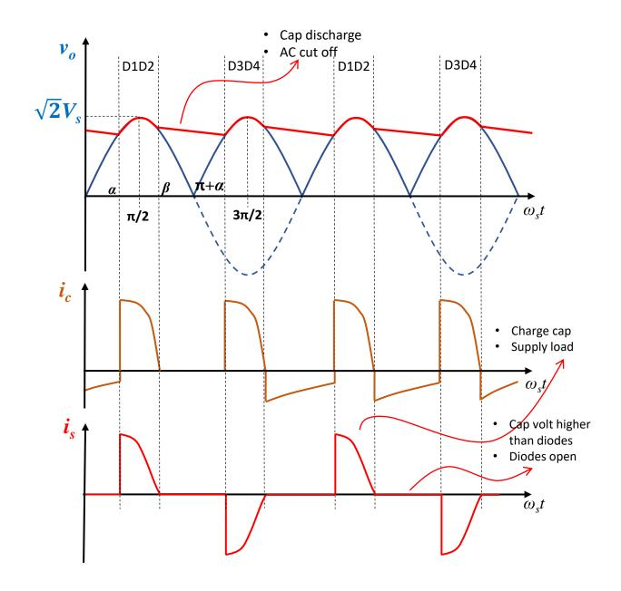
The capacitor is only recharged when the capacitor voltage falls below the input voltage, i.e., when the absolute value of the sinusoidal mains voltage exceeds the capacitor voltage. That leads to very brief current surges around the maximum and minimum of the sine on the mains side, which stresses components and generates high-frequency mains currents.
