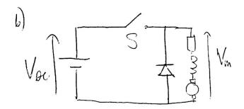
Switch S (MOSFET) a switched on and off with duty cytle  $\rho = Ton/T$ . When on,  $V_m = V_{sec}$ , when off, freewheel diede conducts motor award so  $V_m \sim O$ . Near value of  $V_m$  to  $\rho V_{sec}$  and so armetire voltage can be varied by varying  $\rho$ .
