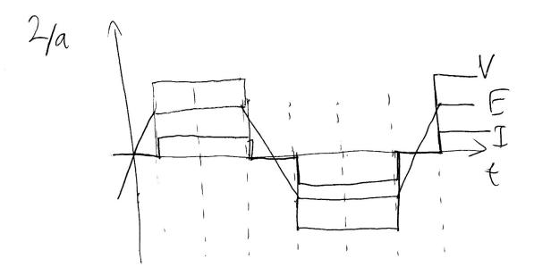
At any teris, two phases conduct, one phase is floating. Hall effect sensors are used to detect the rotar position and hence the phase of the back-cruf. This analls the applied voltage V to be timed so that E e I are in phase (90° torque angle).
