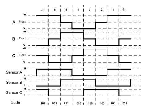
Sensored control is preferred when the drive is required to operate at low speeds and/or has many stop/starts, since back-emf zero-crossing detection is difficult in these cases.
