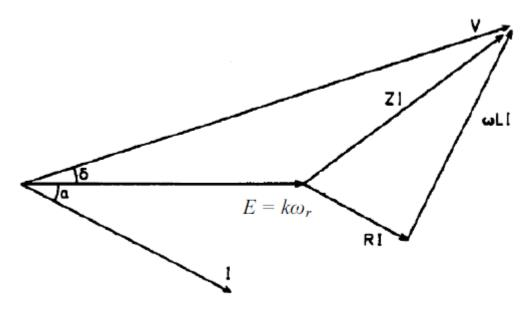
$\delta$  = load angle,  $\delta$ + $\alpha$  = power factor angle, E = induced emf, V = voltage; note: resistance cannot be ignored like sinusoidal BLDCM
