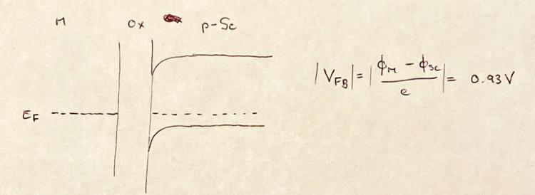
$$V_{T} = -\frac{Q_{D}}{C_{ox}} + V_{S} + V_{FB}$$
