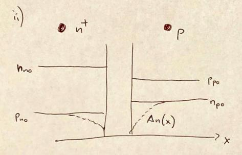
Reverse saturation current dominated by minority carrier extraction and their drift across deplotion region.
