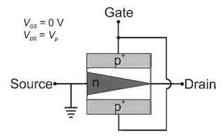
Further increase in  $V_{DS}$  has no significant effect upon  $I_{DS}$ , which remains at its saturated level, and this is called the saturated region. [20%]
