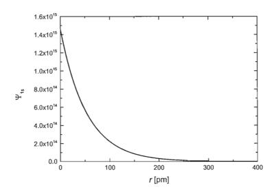
The probability of finding the electron at a particular radius is a little more complex.  $|\Psi_{1s}|^2$  gives the simple probability per unit volume, but we need to consider the volume of a thin shell of space at a radius r as being  $4\pi r^2 dr$ , so that the probability as a function of radius becomes
