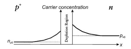
In forward biased p+n junction minority carriers are electrically injected, similar to the optical injection in (a). No electrical fields are assumed outside depletion region, hence master equation and boundary conditions (and hence general solution) are the same for injected holes in n-region and for (a).
