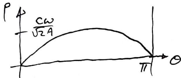
Note that  $\cot \theta = 0$  for  $\theta = \frac{\pi}{2}$  so the  $J$ , term vanishes. This is because nutation around  $\theta = \frac{\pi}{2}$  is not associated with rotation of the assembly about  $k$ .
