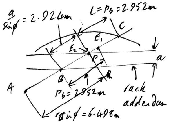
Limits of single pair contact between  $E_1$  and  $E_2$ . Noting that  $L = p_b$ ,  $E_2$  coincides with P.
