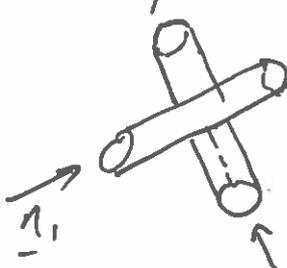
The contact normal for the crossed cylinders setup is normal to the  $\underline{n}$  vectors pointing along the axes of the two cylinders.
