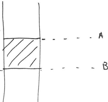
However 3D square mechanism will be shallower than strip. If strength increases with depth, shallow mechanism will utilise lower soil strength leading to lower  $S_c$ .
