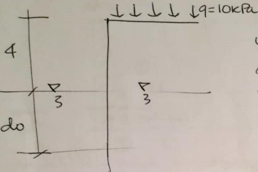
$\phi' = 33^\circ$      $\delta = \frac{1}{3}\phi' = 11^\circ$
