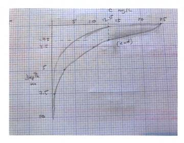
The dispersion curves follows the expected S shaped profile with the 50% concentration at depth of 1.752m. Link this point with the 24.5mg/L concentration at depth zero, roughly and plot the calculation c values at 2.5m, 5m and 7.5m, similar to the diffusion profile. [20%]
