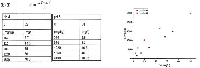
At pH=4, the adsorption isotherm is approximately linear.  $K_d = q/c_e$  which is indicated by the slope of the adsorption curve. So K<sub>d</sub> = 21 L/kg.
