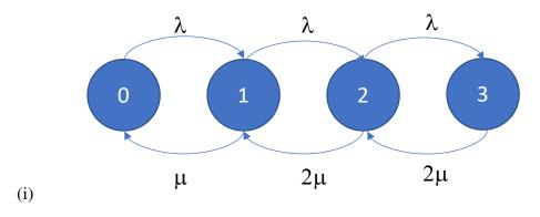
$$\begin{split} \lambda \pi_0 &= \mu \pi_1 \quad \Rightarrow \quad \pi_1 = \lambda / \mu \pi_0 = \rho \pi_0 \\ \lambda \pi_0 + 2\mu \pi_2 &= (\lambda + \mu) \pi_1 \quad \Rightarrow \quad \pi_2 = \rho^2 / 2\pi_0 \\ \lambda \pi_1 + 2\mu \pi_3 &= (\lambda + 2\mu) \pi_2 \quad \Rightarrow \quad \pi_3 = \rho^3 / 4\pi_0 \end{split}$$
