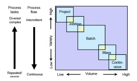
Job shops hence require significantly more effort for sequencing and scheduling jobs than mass production for example. Assignment of labour will be dependent on the work load and there will be a significant need for load balancing of both labour and equipment.
