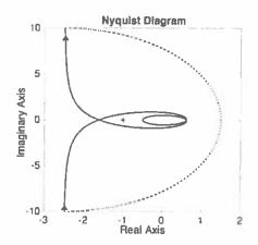
(c.ii) For  $\tau = 3$ , closed loop stability holds for  $K < \frac{1}{1.6}$ . The open loop has no unstable poles therefore, by Nyquist criterion, we search the gain K that guarantees 0 encirclements of the point -1/K. For positive K, 0 encirclements are achieved if
