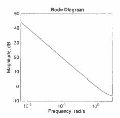
(b.ii) The step responses is unbounded since the magnitude of the Bode diagram goes to infinity when the frequency approaches 0.
