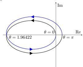
(ii) The open loop system has two poles strictly outside the unit circle, so the closed loop system will need two encirclements of the pont -1/K to achieve stability. This is the case for -1/K between  $H(e^{1.96422j}) = -0.933$  and  $H(e^{0j}) = H(1) = 0$ ,
