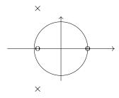
We note that there are 2 poles outside the unit circle so the system is unstable, which was to be expected since it models a continuous time system with negative damping coefficient.
