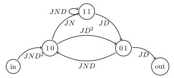
We can now obtain the transfer function either by solving a sytem of equations or using Mason's rule
