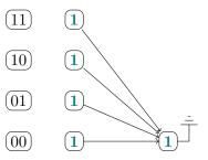
For the summary stage, we only need to compute the  $\alpha_i \gamma_{ij} \beta_j$  for the relevant trellis stage that contains  $U_3$  and  $X_5$ :
