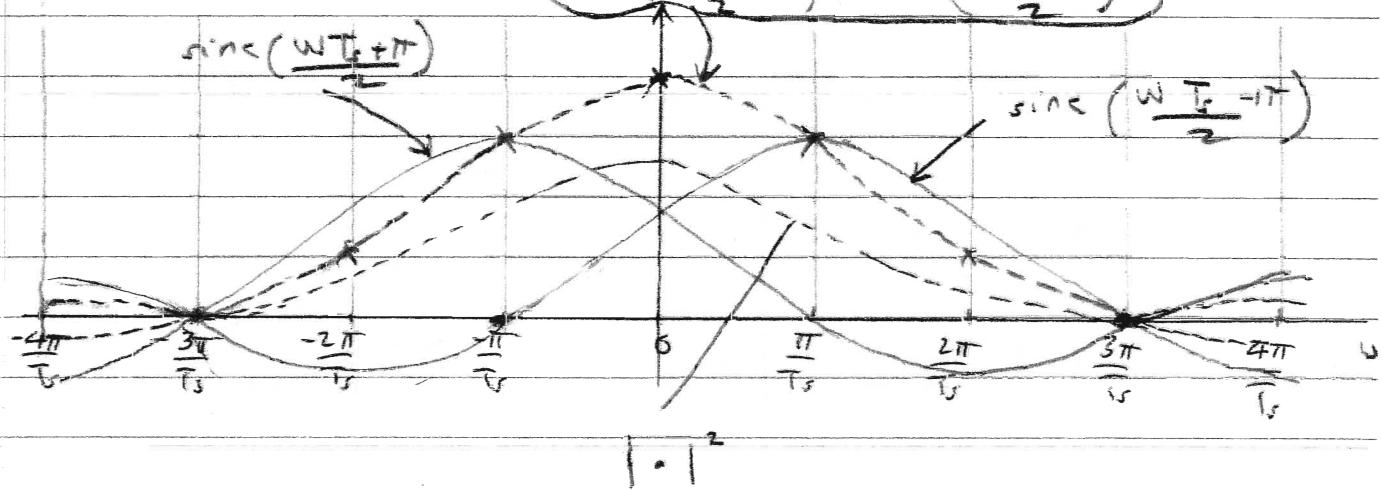
If rectangular pulses of duration  $\pm T_s/2$  are used the resulting sinc frequency response has nulls at  $\omega = \pm \frac{2\pi}{T_s}$ .
