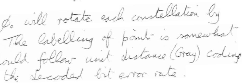
Phase offsets  $\phi_0$  will rotate each constellation by  $\phi_0 \approx 5^\circ$ . The labelling of points is somewhat arbitrary but should follow unit distance (Gray) coding to minimize the decoded bit error rate.
