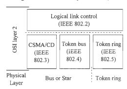
Layer 2 is split into the LLC and the MAC. This was to split the control of the LAN from the media dependant functions. The different types of LAN are characterised by their distinctive topologies. They all comprise a single transmission path interconnecting all the data terminal devices, together with the appropriate protocols (called the logical link control (LLC) and the medium access control (MAC)) to enable data transfer. The LLC and MAC split the data-link layer (Layer 2)
