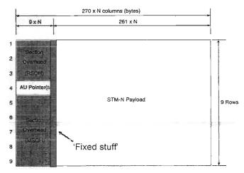
1st basic SDH mux unit is the STM-1 (synchronous transport module) frame which is at a data rate of 155Mbits/sec. STM-1 signal is a repeated series of 125usec frames of 270x9 (2430) bytes. 155Mbit/sec = 243 x 64kbit/sec
