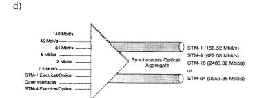
How can we accommodate both voice and data on SDH? SDH has been designed for low latency and minimal delays, which is ideal for voice. The synchronous Mux has been designed with flexibility in mind which allows different data type to ne mapped into STM-N frames with careful management. Data (especially Internet
