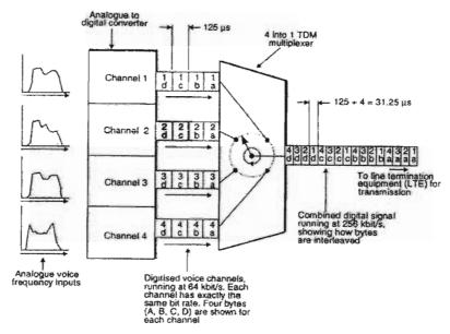
c) The problem occurs when a single 2Mbit channel needs to be dropped or added from a higher order Mux. (Drop and Insert). All of the channels must be demuxed and then muxed again as the position of a channel is unknown in the higher orders. ie 140 to 34, 34 to 8 and then 8 to 2Mbit/sec. This is very expensive as it requires a lot of equipment and invariably leads to delay in any voice services.
