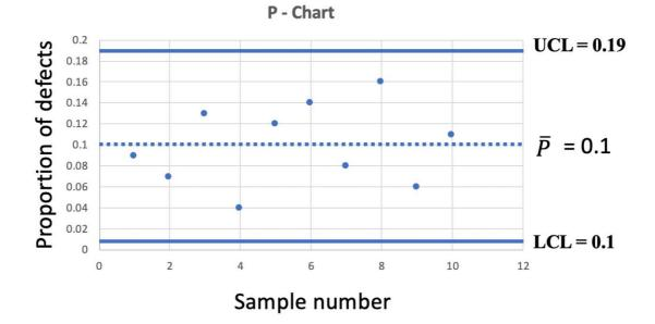
Whilst the process here is shown to be in control, there is still room for improvement. The engineering team should examine the manufacturing processes and employ further control charts to identify the root causes of failure.
