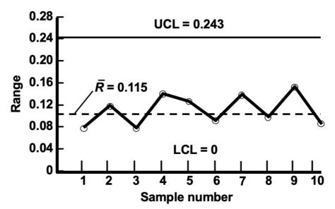
In this case, the sample mean is shifting upward and the range (dispersion) is consistent. This suggests an assignable cause of change which must be investigated further. In order to make a confident purchase, one would need to know the specification limits of the design since these should fall outside of the control limits and hence render the machine suitable for use.
