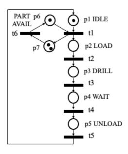
Figure 1 Petri Net of Drilling Operation
