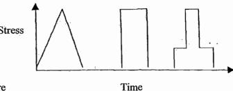
e.g. fast loading may not have the same effect as slow loading; e.g. if the sample is kept under load, it may creep.
