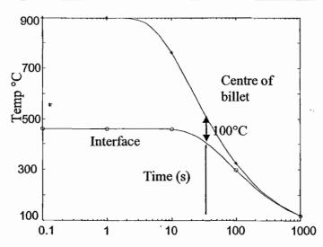
From the graph (more detailed than required), the centre and surface of the billet differ in temperature by 100°C after approximately 35 seconds.
