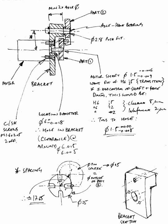
b) With the solution in part (a) in mind, below are the design of two potential components. Specific attention should be given to the 'fit' of the part to the motor shaft and also to the pin in the slot. Marks would be awarded for the precision and clarity of the engineering drawings.
