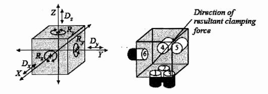
A potential embodiment of a jig design is shown below.
