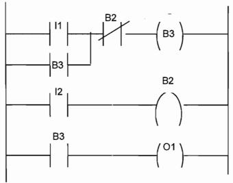
In the above figure, the temporary state B3 is used as a latch for the momentary input I1 that ensures output O1 remains on. B2 is the unlatch function that turns output O1 off, and this is activated by I2
