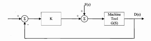
Closing the feedback loop with controller K(s) results in the resulting transfer function from F(s) to D(s) being:
