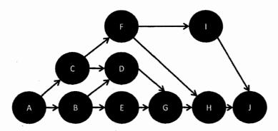
The work content =  $\Sigma p_i$  = 46 minutes Cycle\_time = ((7.5 hours \* 60) - 40) / 36 units = 11.39 minutes/unitMinimum number of stations =  $\Sigma p_i / \text{cycle\_time} = 46/11.39 = 4.04$ , i.e. min. 5 stations.
