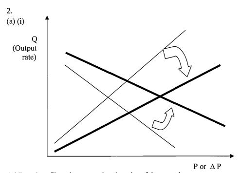
Adding glass fibres increases the viscosity of the extrudate.
