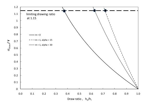
Note that yield at exit is given by  $\sigma_{draw} = \frac{2 Y}{\sqrt{3}}$  (von Mises in plane strain), and not  $\sigma_{draw} = Y$ . Hence drawing limit reached when  $\frac{\sigma_{draw}}{Y} = \frac{2}{\sqrt{3}} = 1.15$
