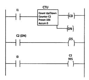
Upward and downward counters are used to monitor the accumulation of events (e.g. parts passing a particular point). Once the accumulated counter reaches the preset value the rung (DN) becomes "true" or "on" and can be used as an alarm or as part of a resetting sequence. CD indicates that the counter is counting.
