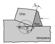
c) Forces acting on the tool face can be developed from the following figure
