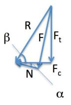
Where  $\begin{aligned} F &= F_c \sin \alpha + F_t \cos \alpha \\ N &= F_c \cos \alpha - F_t \sin \alpha \end{aligned}$
