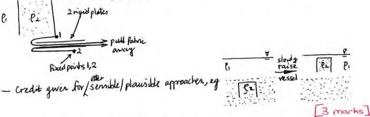
(b) Initial/base state is top heavy, the stabilising effect of surface tension dominates the destabilising effect of buoyancy force. Surfackant would reduce surface tension — disturbances present in base state could grow to produce standing wowers on interface (eg mode shown left) if growth saturated or continued growth could result in fushing of liquida from the venel (right)
